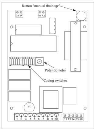
The steam output can be set step less from 20 % to 100 % capacity. For setting the output limitation the electric compartment must be opened and the potentiometer on the electronic print must be adjusted. Turning clockwise increases the steam output and turning anticlockwise reduces the steam output. The output ex works is set at 100 %.
